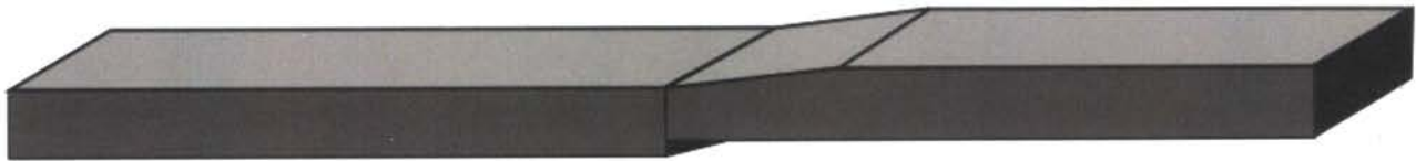
Trip hazard AFTER repair
