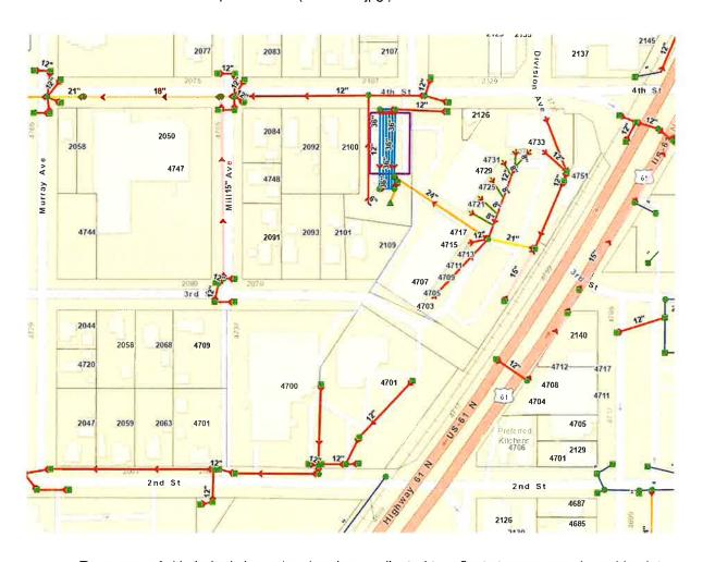
**Response 1:** Hydrologic boundary has been adjusted to reflect storm sewers in parking lot, southwest of Hwy 61 and 4th St interchange and adjusted parcels accordingly. Stormwater from this area flows west to vault under parking lot in VLAWMO. The legal boundary was reverted to its original boundary along US 61, following the hydrologic boundary.
