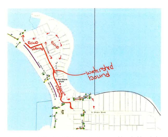
**Response 2:** HEI reviewed LiDAR data and local imagery and determined the revised hydrologic boundary as shown in above image. Hydrologic and legal boundaries have been updated accordingly.
