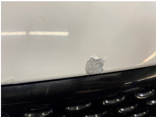
Aluminum corrosion on the front lip of the hood
