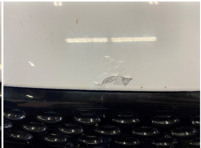
Aluminum corrosion on the front lip of the hood
