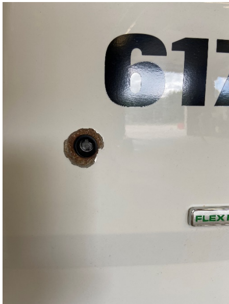
Rust around the keyhole on the rear hatch. Front Driver's door panel is separated and coming apart
