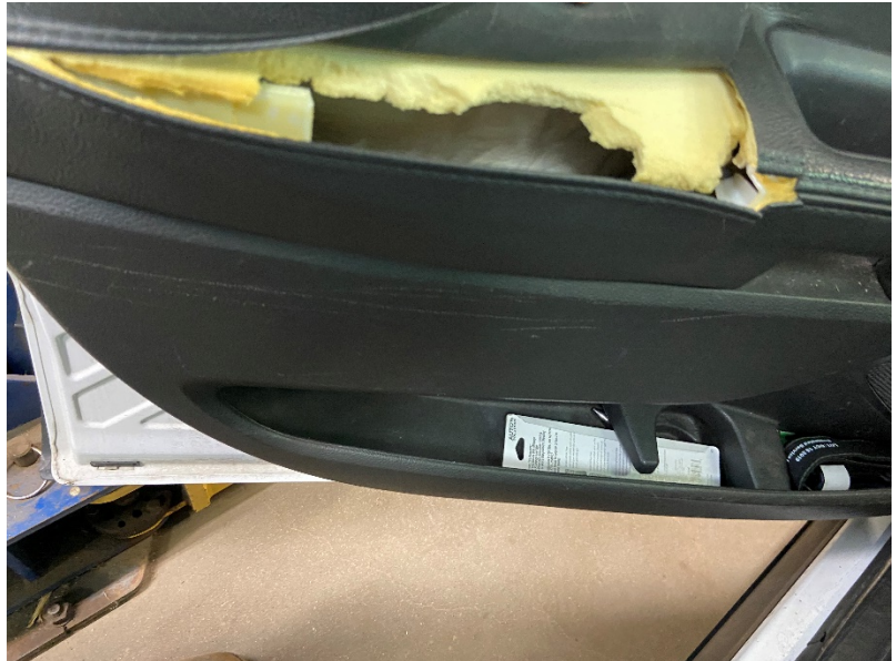
Rust around the keyhole on the rear hatch. Front Driver's door panel is separated and coming apart
