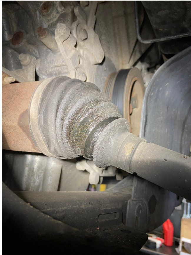
#399 has a leaking front right CV shaft that is in need of replacement.
