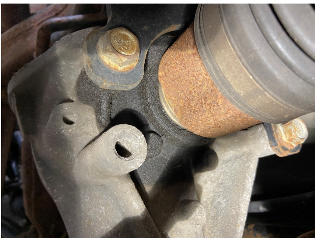
Both axle seals on the rear differential are leaking and should be replaced
