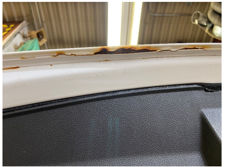
Rust starting on the inside of the rear doors and the bottom lip of the hatch
