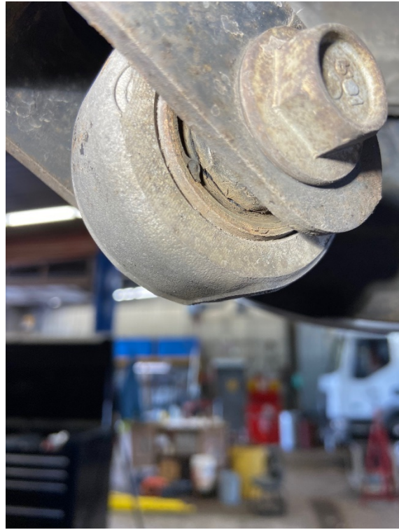
#399 has several rubber bushings on steering/suspension components that are cracked and in need of replacement. This wear is common among our older squad cars due to years of aggressive driving.
