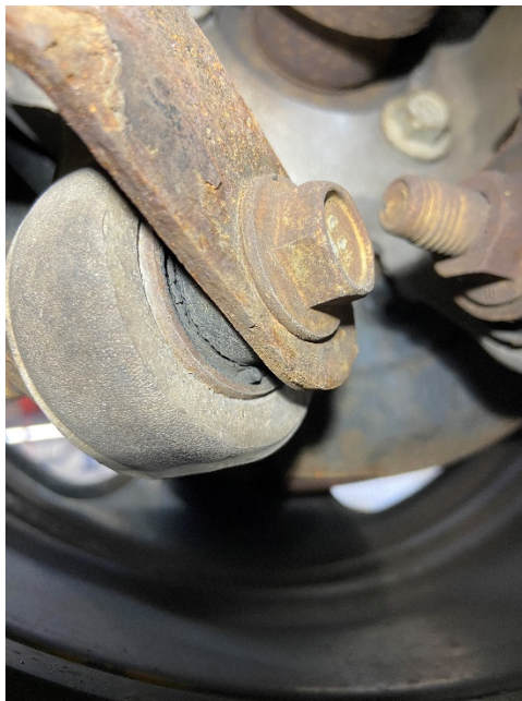
The rear trailing arm bushings are worn and in need of replacement.
