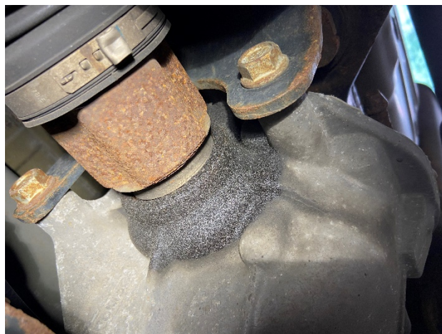
Both axle seals on the rear differential are leaking and should be replaced
