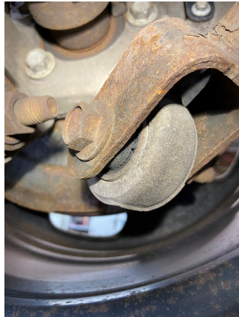
The rear trailing arm bushings are worn and in need of replacement.
