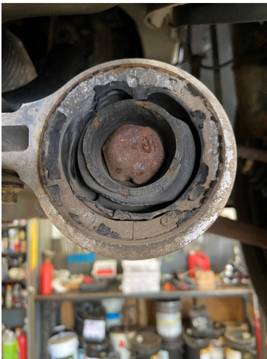
Front lower control arm bushings should be replaced
