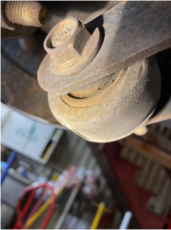
#399 has several rubber bushings on steering/suspension components that are cracked and in need of replacement. This wear is common among our older squad cars due to years of aggressive driving.
