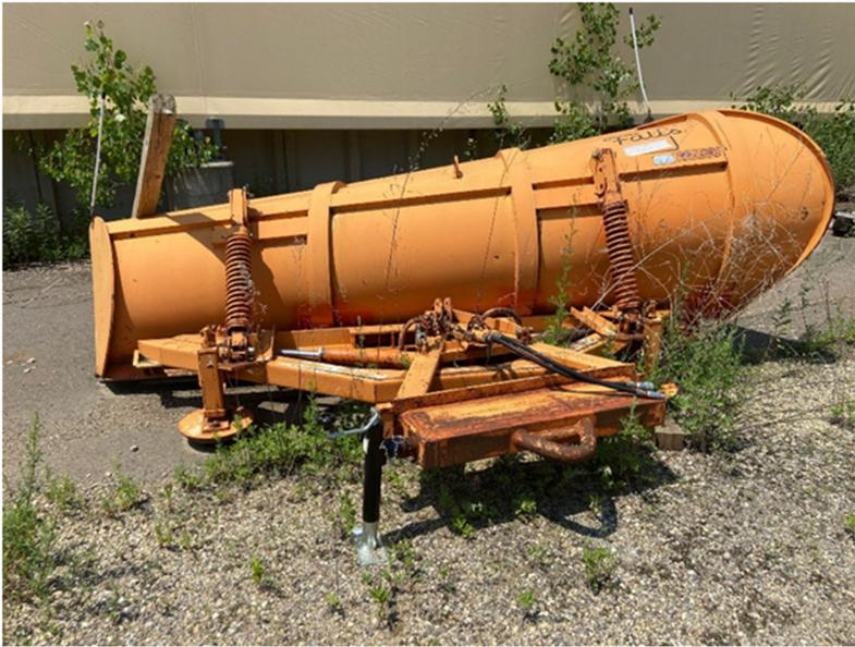
Vehicle #200 was ordered back in 2007 with a single direction highway plow. This plow works fine for plowing highways but it lacks the flexibility to push snow forward and clean cul-de-sacs effectively. It does not carry/push snow forward or allow the driver to put snow to their left hand side. The other four large plow trucks all have reversible plows that allow a lot more flexibility for the driver in neighborhoods, cul-de-sacs and streets lined with parked cars.
