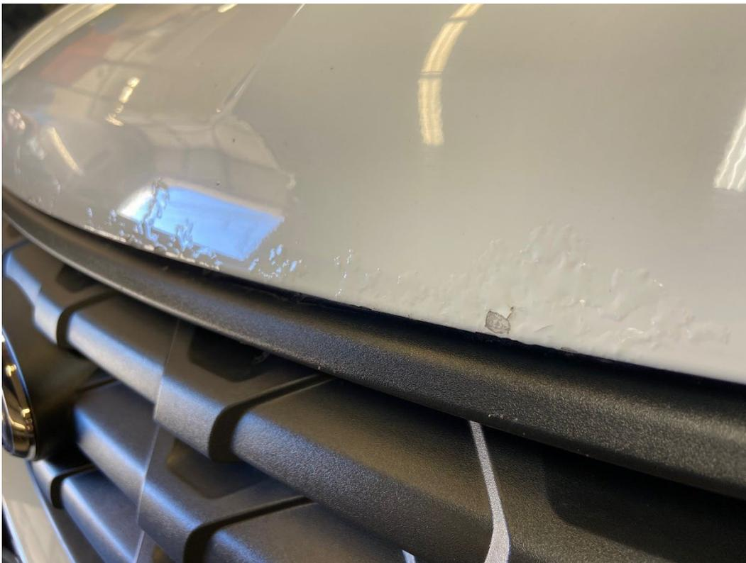
The front edge of the aluminum hood is starting to corrode and the paint will soon start flaking off. This is something that will continue to get worse. If the vehicle is going to be left in the fleet we should try to get a price on a new hood.
