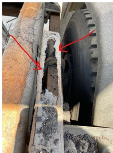
The safety support stand for the hydraulic dump box has completely rusted through. It is meant to support and keep the box from potentially crushing somebody that is working on the truck if the hydraulics for the dump box were to fail. This is used while the box is up in the air and the truck is being worked on.
