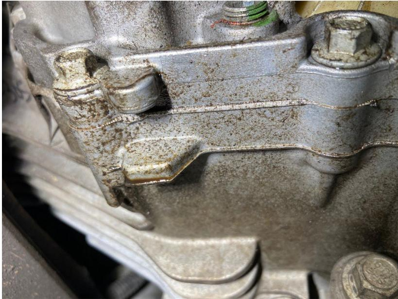
It has a small leak from the PTU (Power Takeoff Unit). It is currently a fairly minor leak but if it needs to be replaced in the future it will be around \$2,500.
