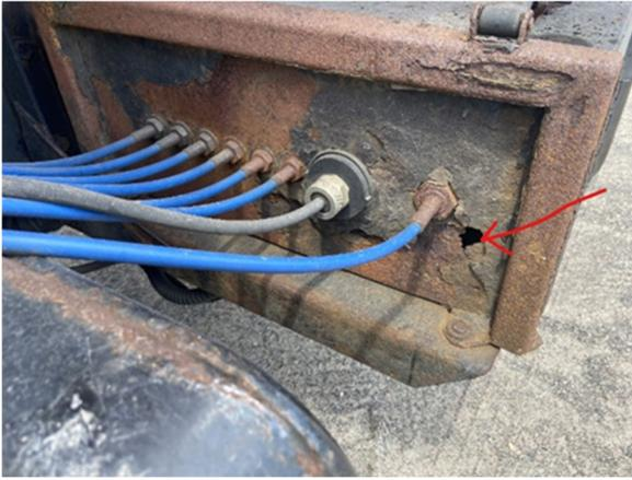
The valve box that contains the expensive hydraulic valves for all of the snow plow hydraulics is extremely rusty and has holes in it. These holes allow dirt, debris and salt to get on to the expensive hydraulic components. The metal is too rusty to attempt to weld/repair and the entire valve box would need to be replaced.
