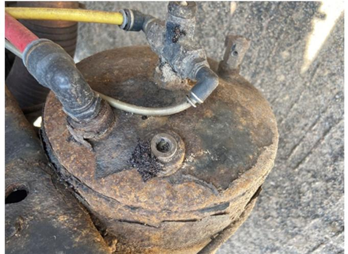
Here are a couple pictures of more extremely rusted components on Vehicle #200. The first picture is of a steel frame pocket that has completely rusted through. The second picture is a picture of the air tank that stores the compressed air that runs the air brakes.
