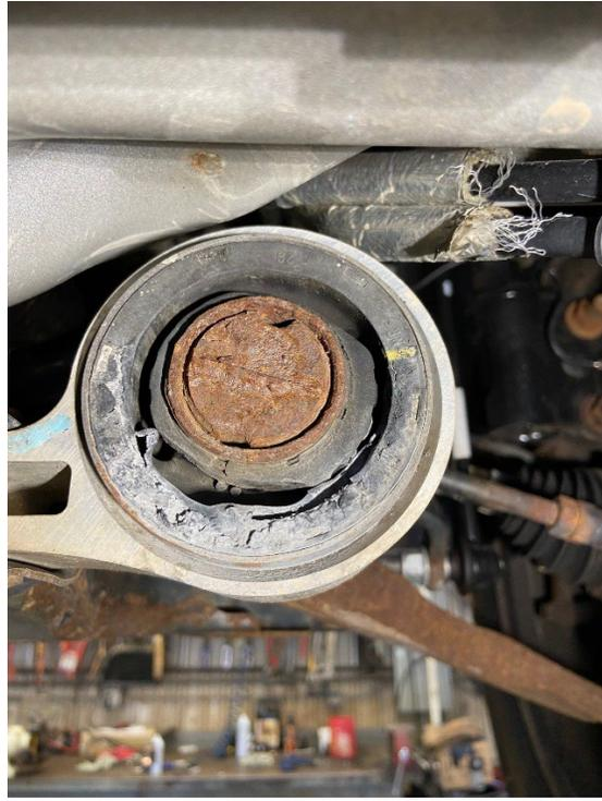
The bushings for the front lower control arms are in rough shape. Both front lower control arms should be replaced.
