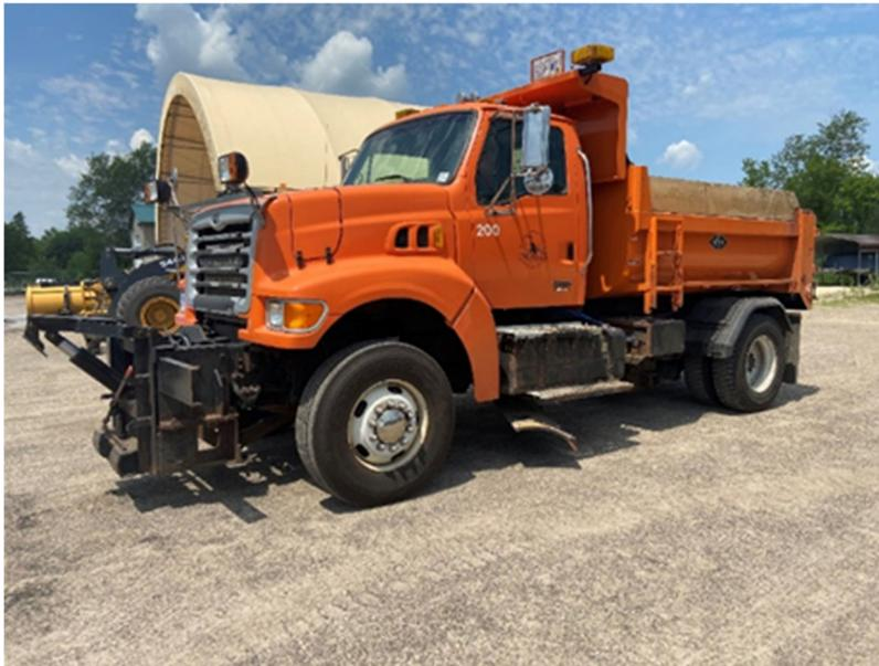
Vehicle #200 is a 2007 Sterling L8500 dump truck. This is our oldest and most often used plow truck. This truck will be 16 years old in 2023 which exceeds the anticipated useful life of a dump truck, which is currently set for 13 years. All of those years of spreading salt has taken a toll on the truck's components.
