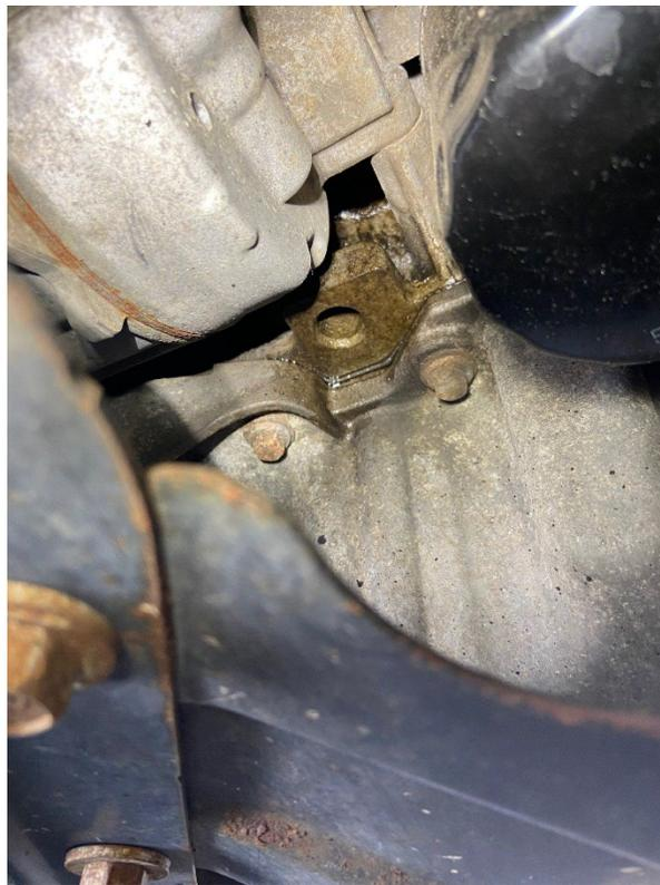
The engine has a small coolant leak, most likely from the water pump. Replacing the water pump is a costly and time consuming repair that requires removing the engine.
