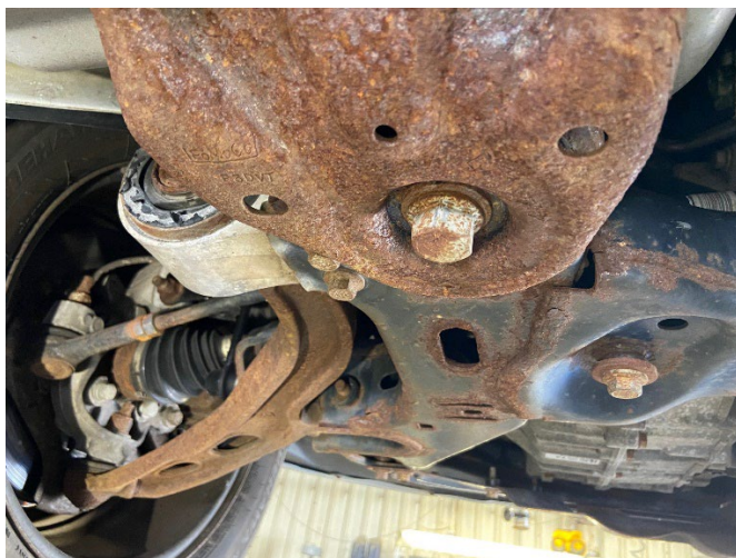
The underside of the vehicle body is showing considerable rust.
