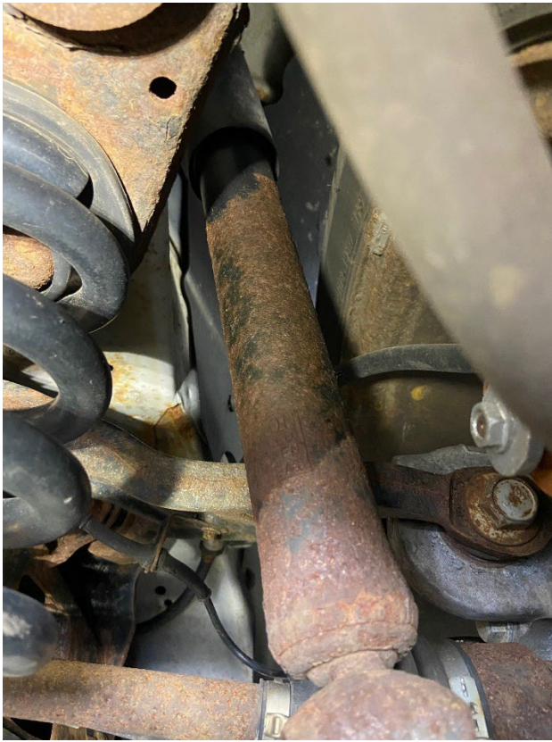
Both rear struts are leaking and in need of replacement.
