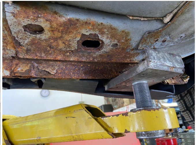
The underside of the vehicle body is showing considerable rust.
