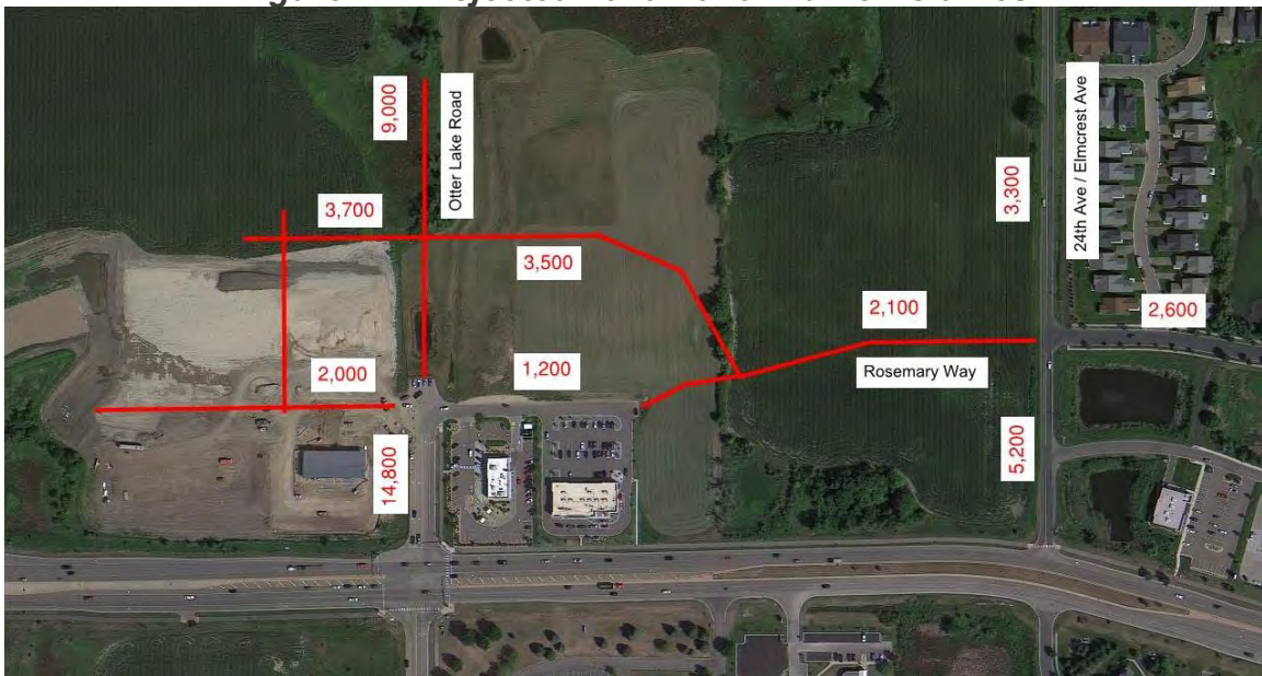
Figure 4 – Projected 2040 Build Traffic Volumes
