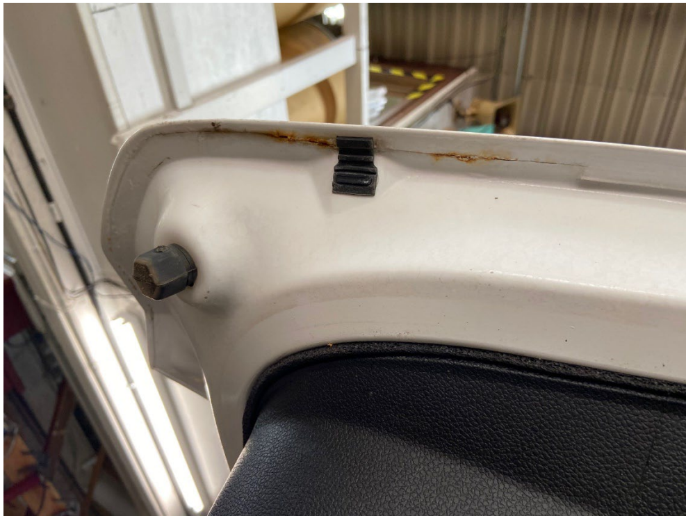
A very small amount of rust is just starting on the inside lip of the tailgate/hatch.
