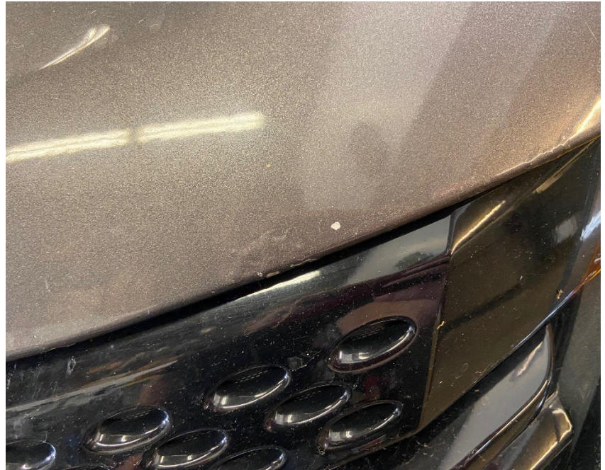
The paint is cracked around the lock cylinder on the tailgate/hatch and will likely start rusting soon. There is also a small amount of corrosion starting on the front lip of the aluminum hood.
