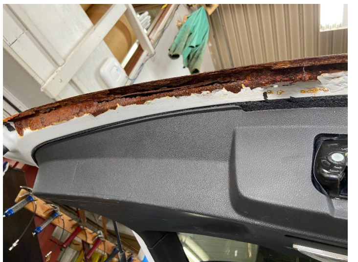
The rear tailgate/hatch is in horrible condition and is in desperate need of replacement.
