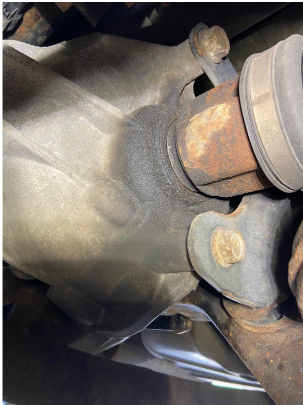
There is a small seep/leak from both axle seals on the rear differential.
