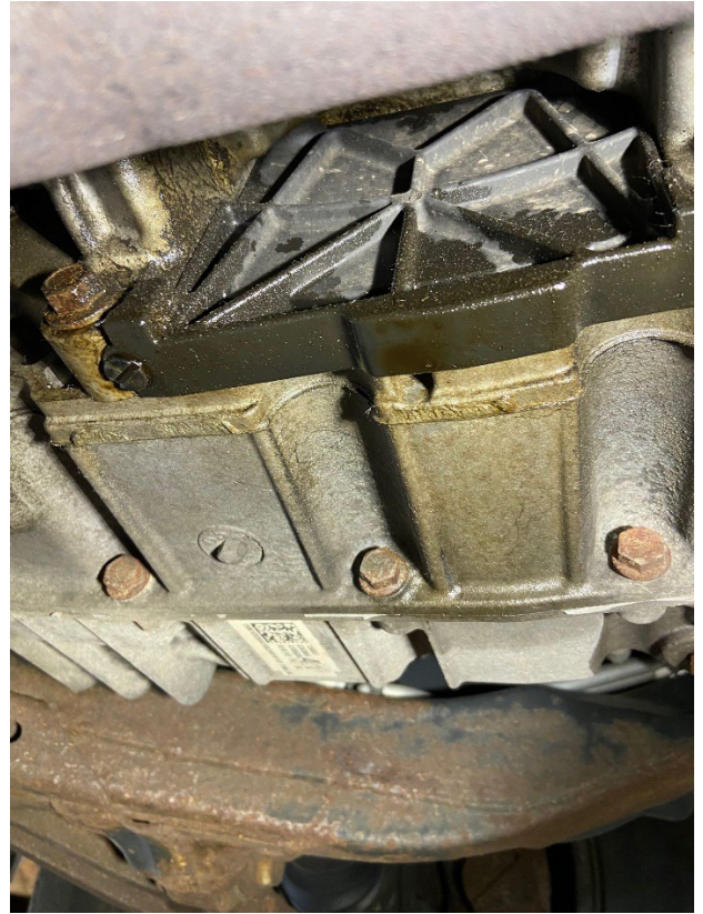
The rear main seal on the engine is leaking engine oil and should be replaced.
