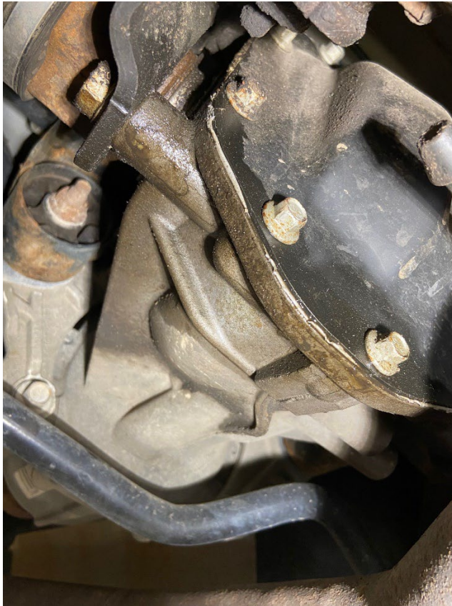
Both axles seals on the rear differential are leaking and in need of replacement.
