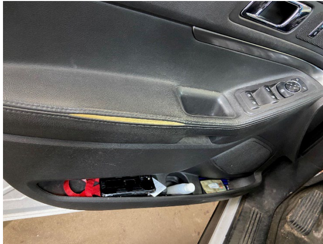
The door panel on the front driver's door is splitting open and in need of replacement.
