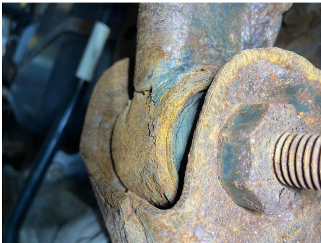
The majority of the rubber bushings on the vehicle are cracked and worn.
