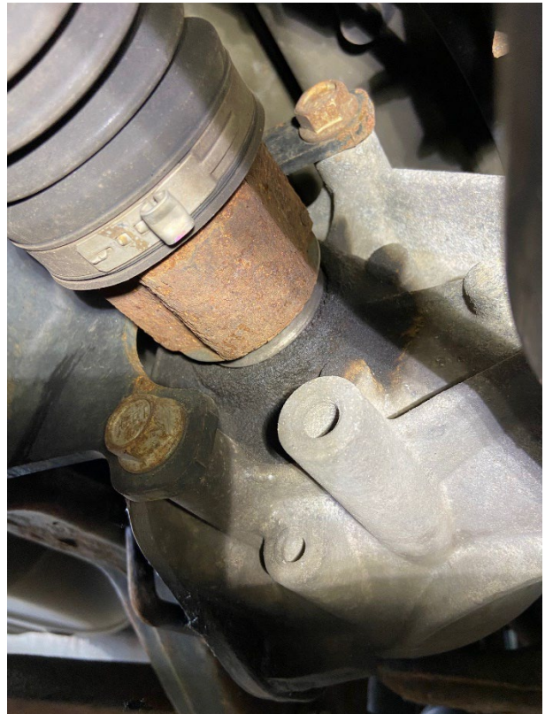
There is a small seep/leak from both axle seals on the rear differential.
