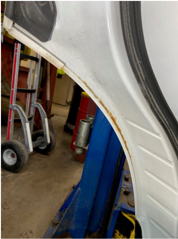
Rust is starting on the inside lip of both rear doors.
