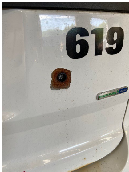
The aluminum hood is showing quite a bit of corrosion. There is also quite a bit of rust forming around the lock cylinder on the tailgate/hatch of the vehicle.
