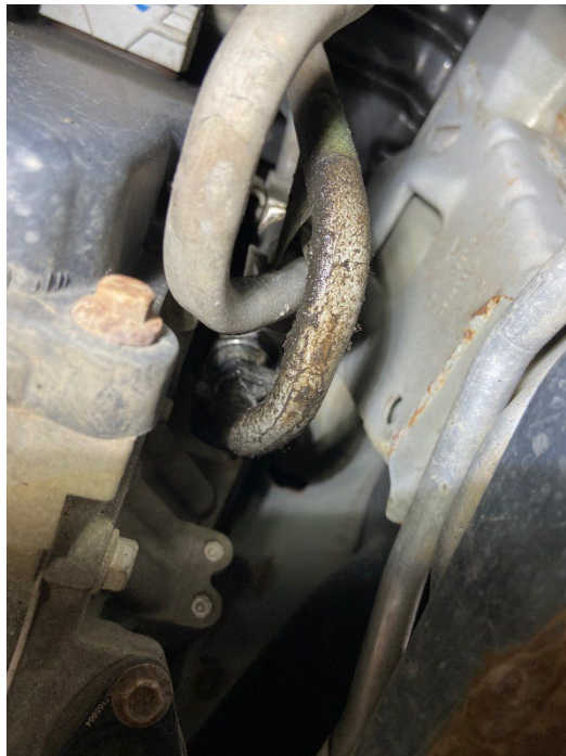
One of the PTU cooler lines is leaking and in need of replacement.
