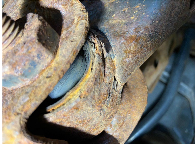
The majority of the rubber bushings on the vehicle are cracked and worn.
