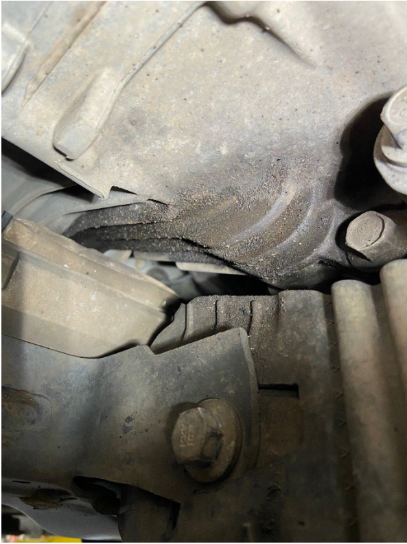
The output seal on the back of the PTU is leaking and should be replaced.
