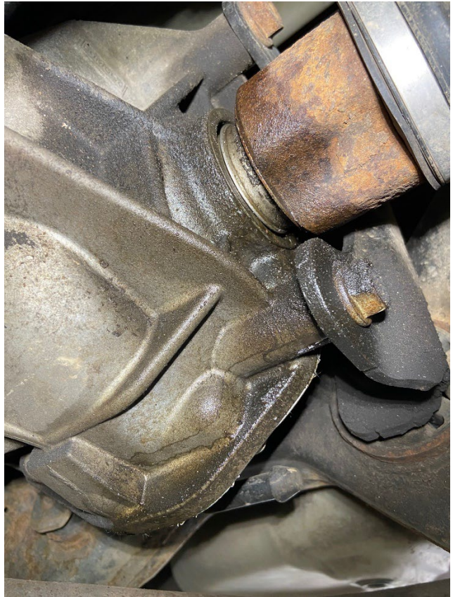
Both axles seals on the rear differential are leaking and in need of replacement.
