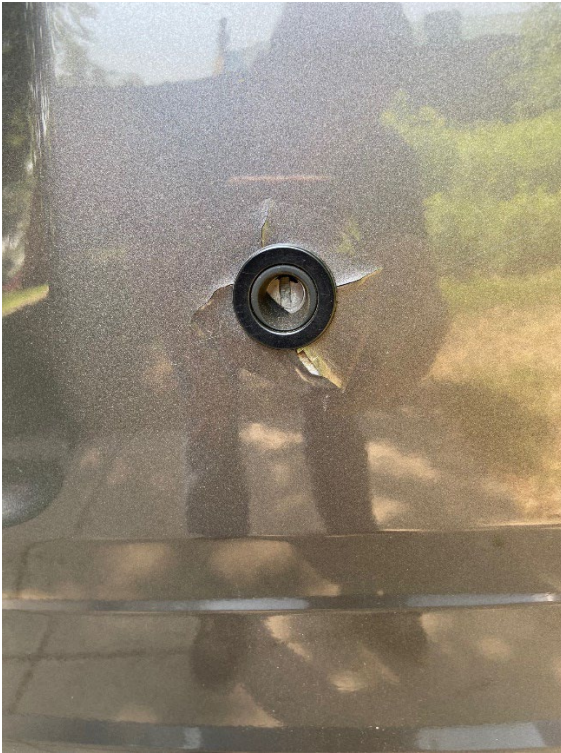
The paint is cracked around the lock cylinder on the tailgate/hatch and will likely start rusting soon. There is also a small amount of corrosion starting on the front lip of the aluminum hood.
