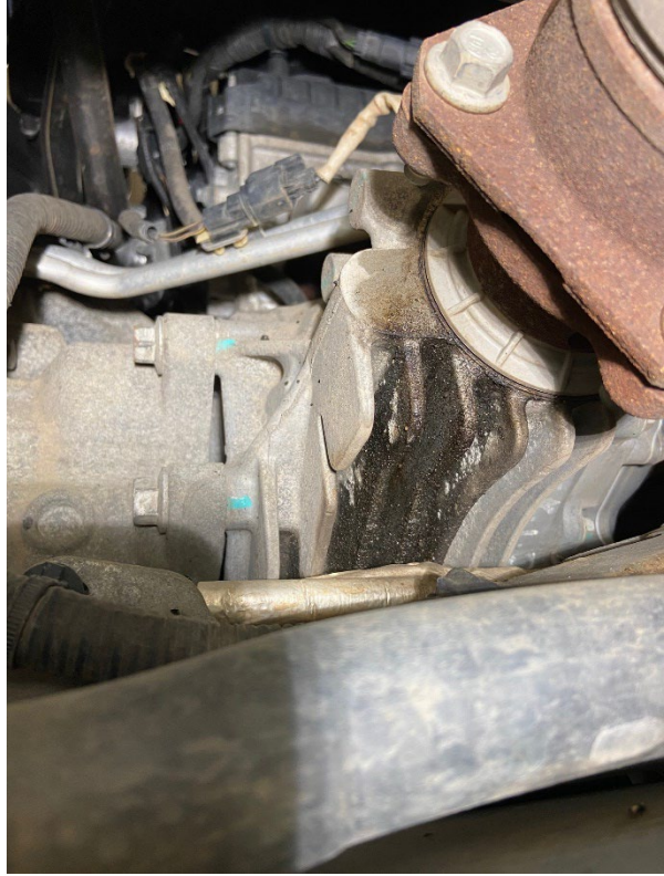
The output seal on the back of the PTU is leaking and should be replaced.
