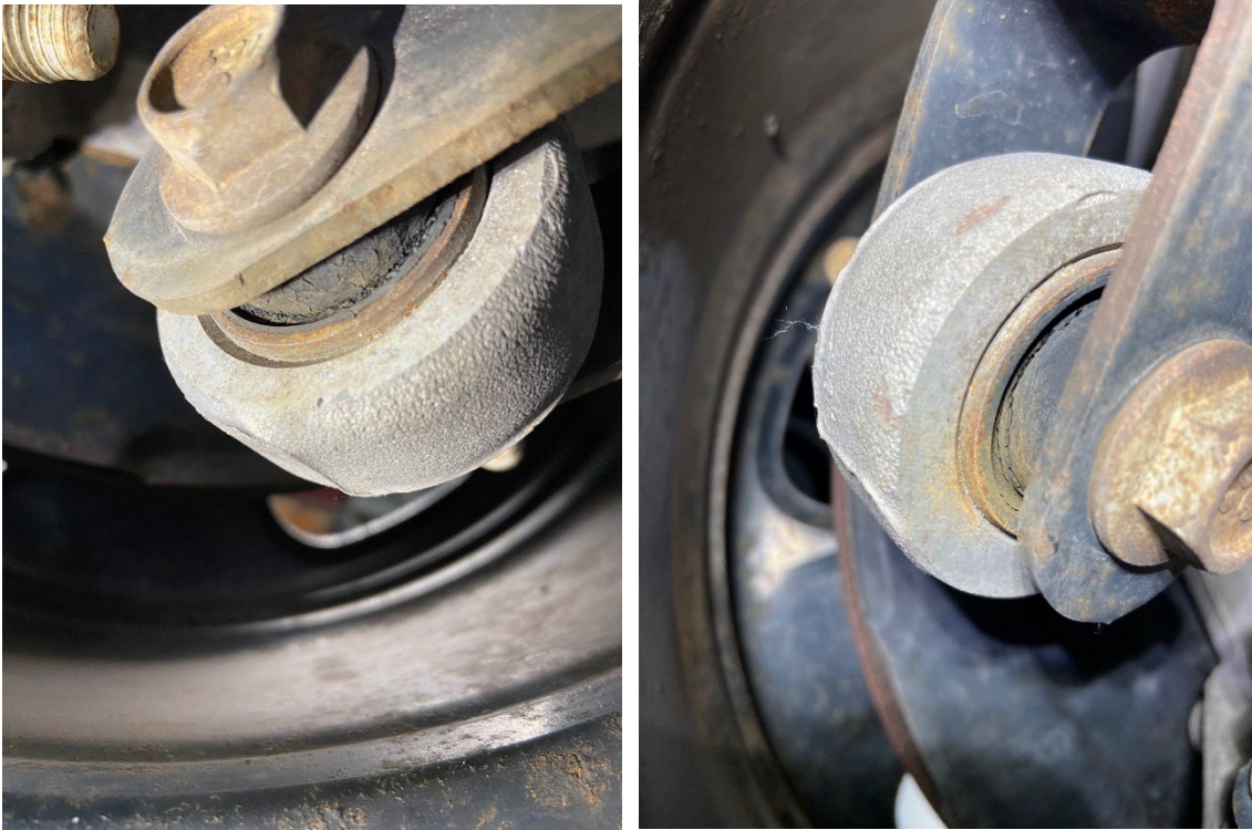
Various rubber bushings are cracked and worn.
