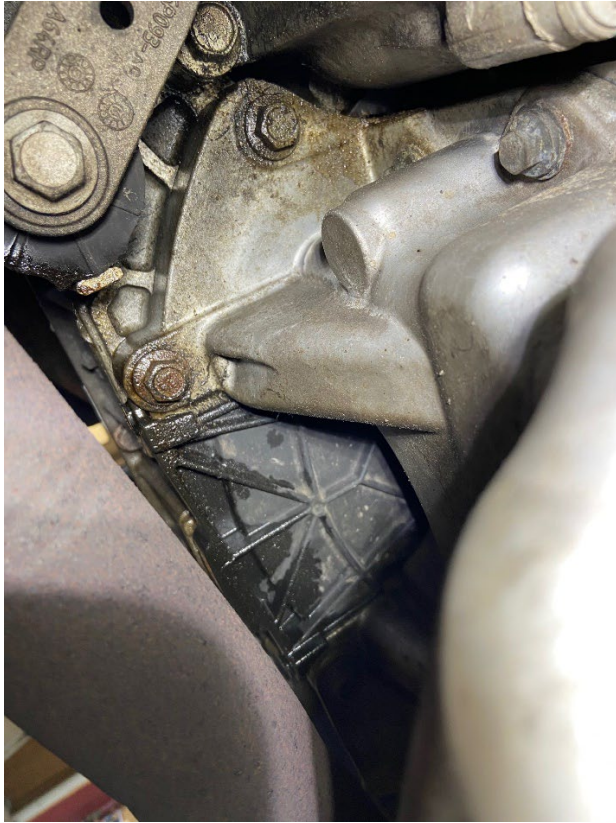
The rear main seal on the engine is leaking engine oil and should be replaced.
