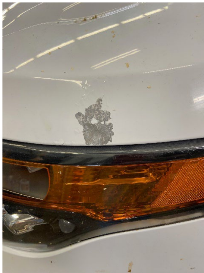
The aluminum hood is showing quite a bit of corrosion. There is also quite a bit of rust forming around the lock cylinder on the tailgate/hatch of the vehicle.
