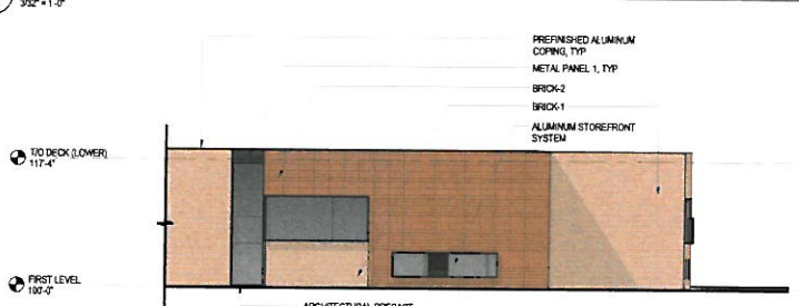
4F ELEVATION - SOUTH (CLASSROOM POD) - DESIGN DEVELOPMENT 3/32" = 1'-0"
