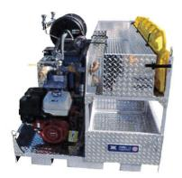
Add a 4' cross lay tray (pre-connect) to hold booster line and one open toolbox holder to carry long tools with holder for long board on passenger side of skid unit
