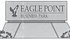
SECONDARY PROJECT IDENTIFICATION: Painted cement base, painted aluminum cabinet with cut through letters. Black letters during day; white illuminated letters at night. Approximately 7' high X 12' wide
