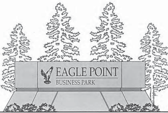
PRIMARY PROJECT IDENTIFICATION: Stone base, painted aluminum cabinet with cut through letters. Black letters during day; white illuminated letters at night. Approximately 15' high X 25' wide
