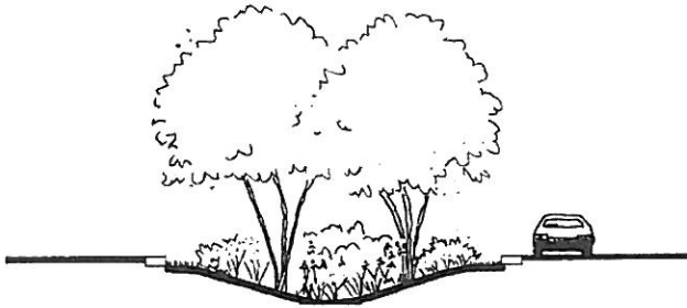
Cul-de-sac infiltration island accepts stormwater from surrounding pavement.
