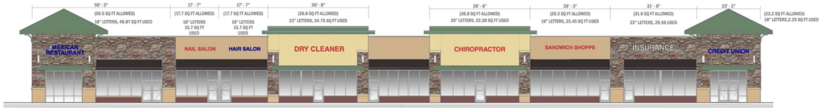
1 PROPOSED: NORTH ELEVATION (FRONT), ILLUMINATED CHANNEL LETTERS. 5" RETURNS, 1" TRIMCAP, 3/16" ACRYLIC FACES. 1 SCALE: 1"=20'-0"
