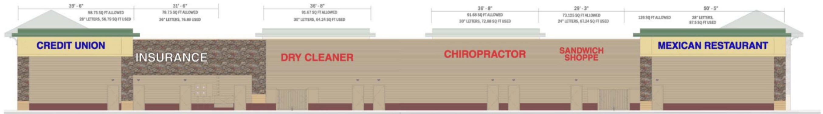
2 1 PROPOSED: SOUTH ELEVATION (BACK), ILLUMINATED CHANNEL LETTERS. 5" RETURNS, 1" TRIMCAP, 3/16" ACRYLIC FACES. SCALE: 1"=20'-0"
