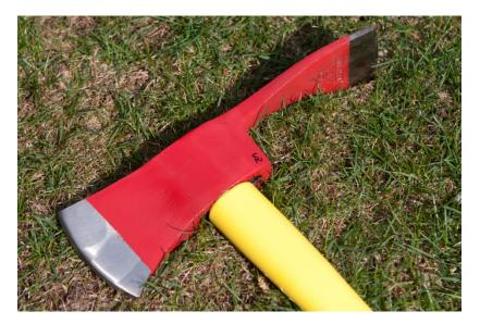
Pulaski: ax-type tool used for chopping small stumps and roots out of the trail tread.
