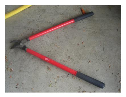
**Pruner:** Cutting tool used for cutting small branches and saplings.
