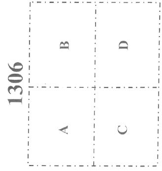
This city block is divided by property lines, the four existing buildings have different owners. If building "A" changes its use and meets the thresholds in 1306, building "A" would be required to be sprinklered, buildings "B", "C", and "D" would not.
