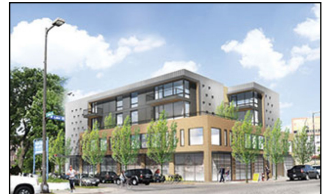
Building Mass is reduced by breaking the building up into smaller sections and “stepping-back” levels above the ground floor. Source: www.minnpost.com
