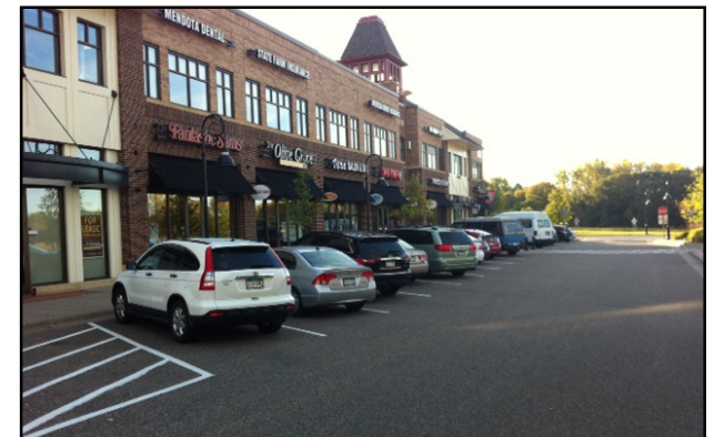
Angled parking promotes traditional main-street character and provides a greater buffer between pedestrian and automobile areas.
