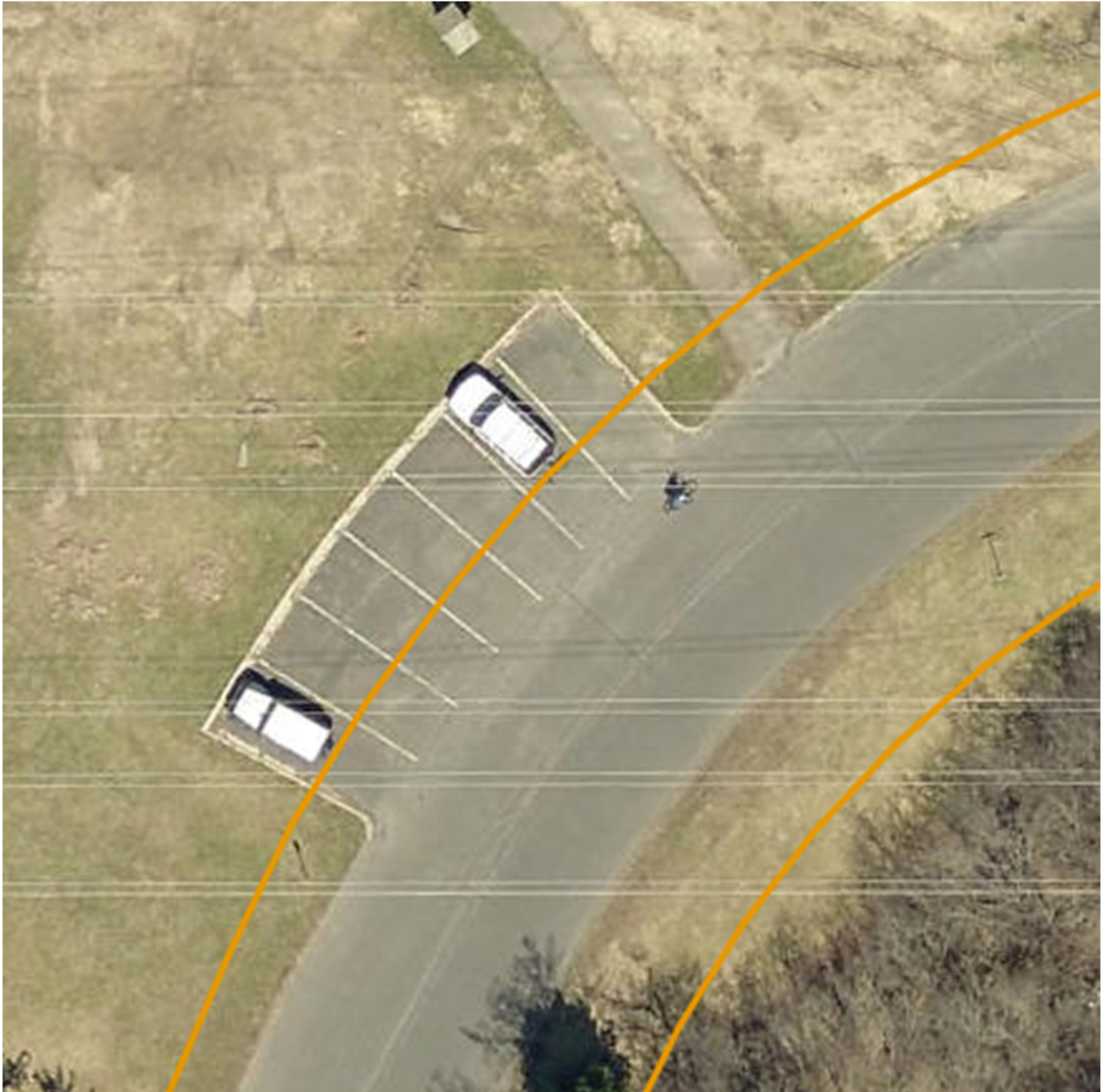
Hytrail Ave Parking Lot: Six 4" SW stripes at 25 ft long
