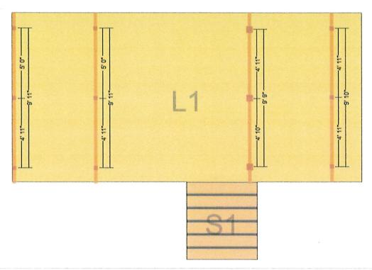
Dimensions displayed are from center of post to center of post.
