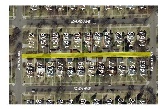
The proposed project involves storm water utility work, small adjustments to the road elevation of the eastern portion of the alleyway, and milling and overlaying the pavement on the entire length of the alleyway. This project is proposed to address the drainage issue on the eastern end of the alleyway and also to improve the pavement condition over the entire length of pavement.
