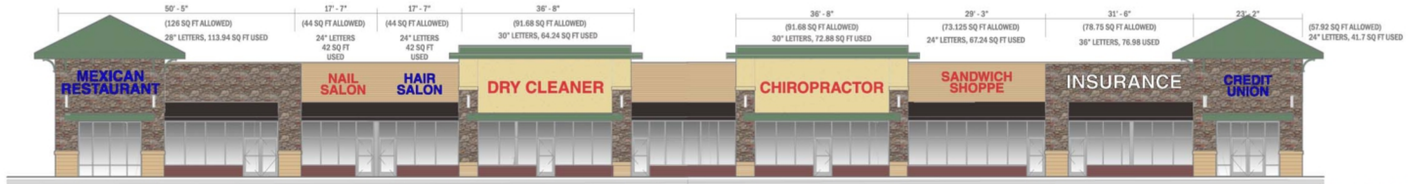
1 1 PROPOSED: NORTH ELEVATION (FRONT), ILLUMINATED CHANNEL LETTERS. 5" RETURNS, 1" TRIMCAP, 3/16" ACRYLIC FACES. SCALE: 1"=20'-0"
