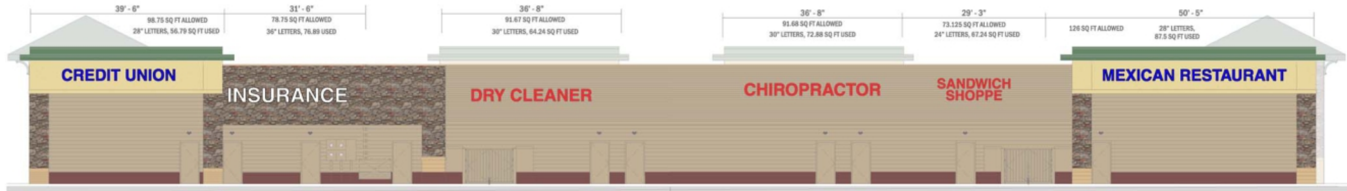
2 1 PROPOSED: SOUTH ELEVATION (BACK), ILLUMINATED CHANNEL LETTERS. 5" RETURNS, 1" TRIMCAP, 3/16" ACRYLIC FACES. SCALE: 1"=20'-0"
