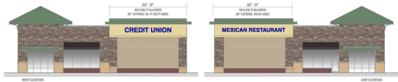
3 1 PROPOSED: WEST & EAST ELEVATIONS, ILLUMINATED CHANNEL LETTERS. 5" RETURNS, 1" TRIMCAP, 3/16" ACRYLIC FACES. SCALE: 1"=20'-0"
