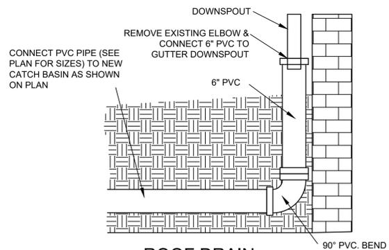
**ROOF DRAIN CONNECTION DETAIL**
