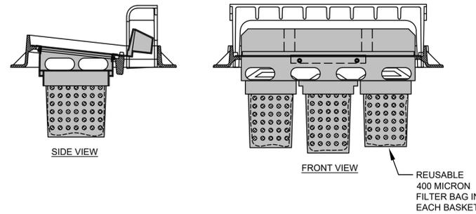
**INFRASAFE INLET PROTECTION DEVICE (OR EQUAL)**
