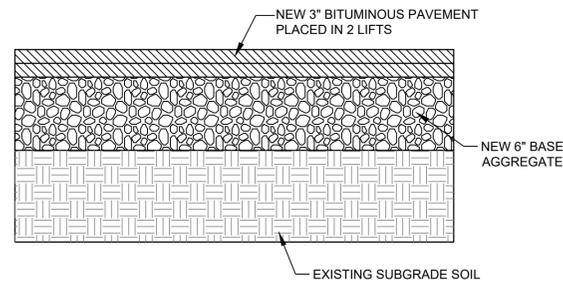
**LIGHT-DUTY BITUMINOUS PAVEMENT SECTION**
