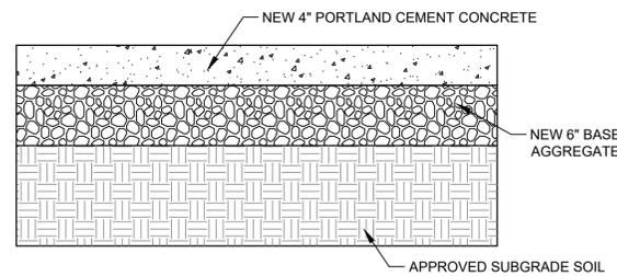
**CONCRETE SIDEWALK CONSTRUCTION DETAIL**
