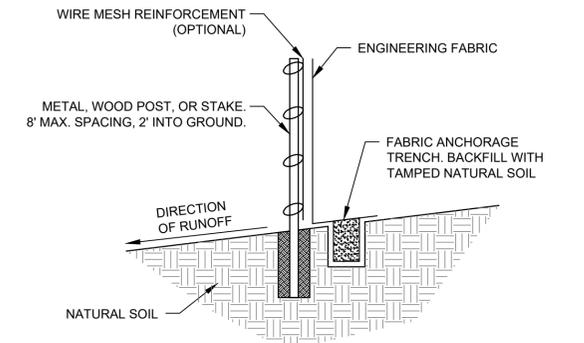
**SILT FENCE INSTALLATION DETAIL**
