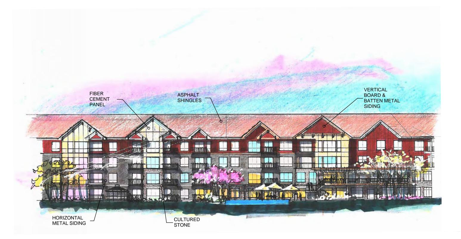
EAST ELEVATION AT POOL AND DECK AREA
