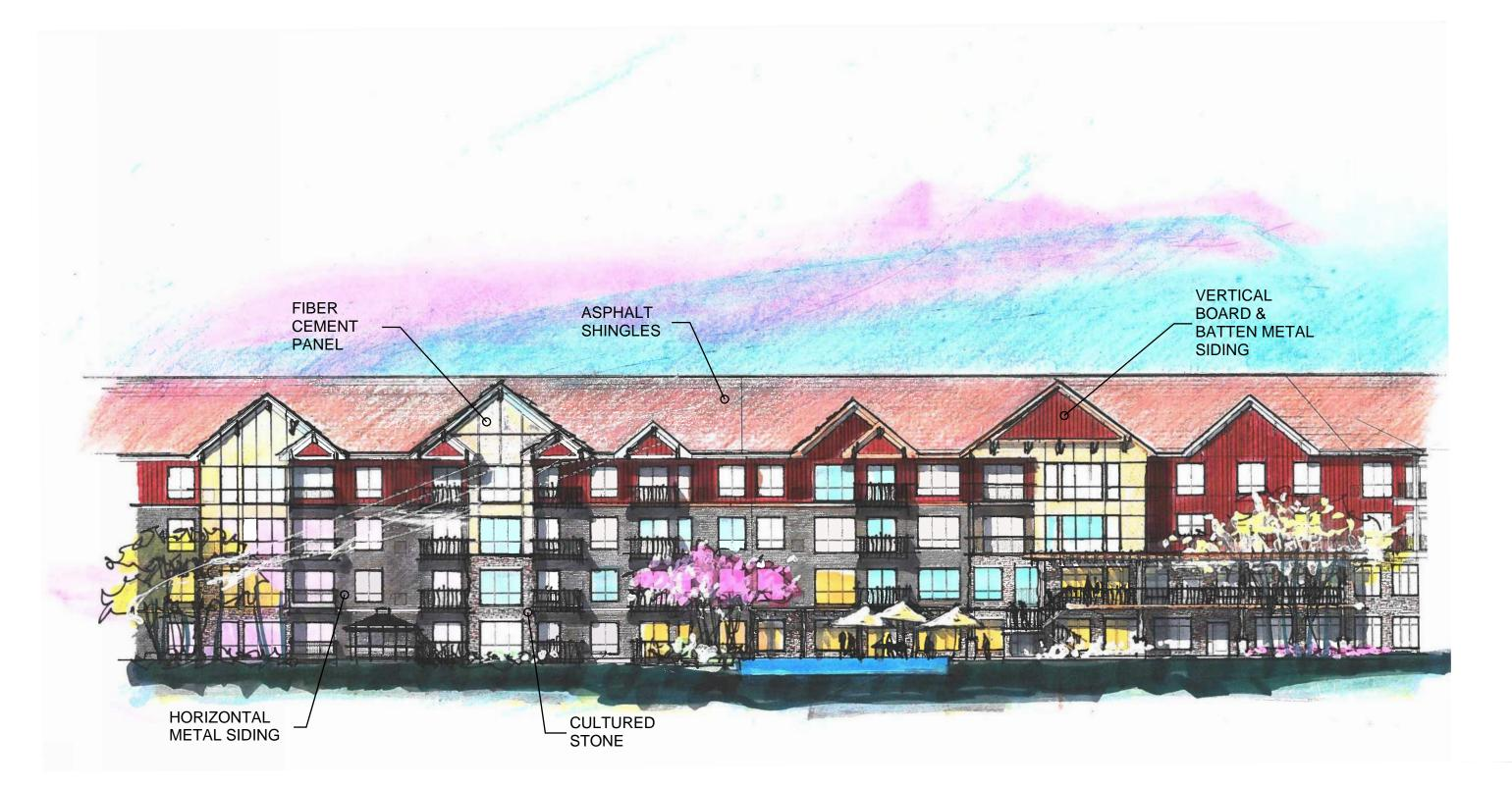
EAST ELEVATION AT POOL AND DECK AREA
