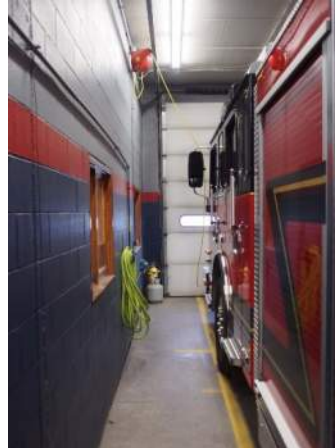
Figure FS1-H.1: Insufficient space in apparatus bays
