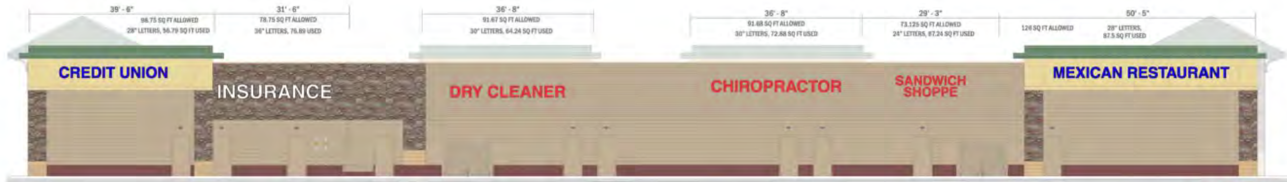
2 1 PROPOSED: SOUTH ELEVATION (BACK), ILLUMINATED CHANNEL LETTERS. 5" RETURNS, 1" TRIMCAP, 3/16" ACRYLIC FACES. 2.5X PER LF OF FRONTAGE SCALE: 1"=20'-0"
