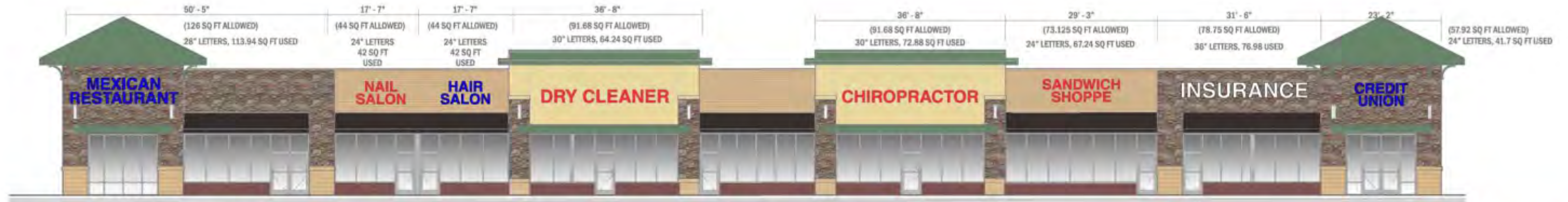
1 1 PROPOSED: NORTH ELEVATION (FRONT), ILLUMINATED CHANNEL LETTERS. 5" RETURNS, 1" TRIMCAP, 3/16" ACRYLIC FACES. 2.5X PER LF OF FRONTAGE SCALE: 1"=20'-0"
