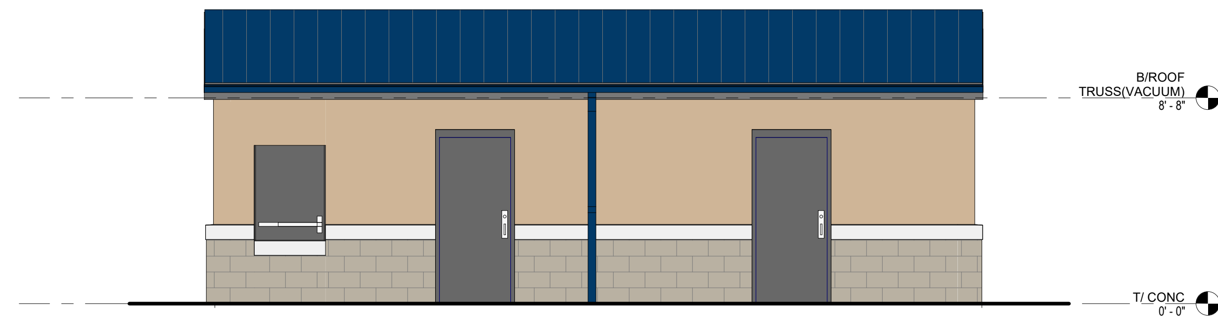
6 A804 VACUUM BUILDING ELEVATION 2 1/4" = 1'-0"
