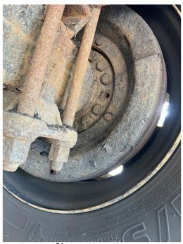
The left rear brake shield has completely rusted off of the truck and the right side is not too far behind. This is not a serious failure but it is an example of the amount of rust and corrosion that this vehicle sees on an annual basis.
