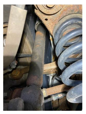
Both rear struts are leaking and in need of replacement.
