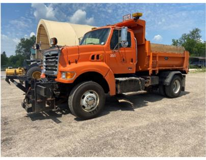
Vehicle #200 is a 2007 Sterling L8500 dump truck. This is our oldest and most often used plow truck. This truck will be 16 years old in 2023 which exceeds the anticipated useful life of a dump truck, which is currently set for 13 years. All of those years of spreading salt has taken a toll on the truck's components.
