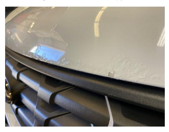
The front edge of the aluminum hood is starting to corrode and the paint will soon start flaking off. This is something that will continue to get worse. If the vehicle is going to be left in the fleet we should try to get a price on a new hood.
