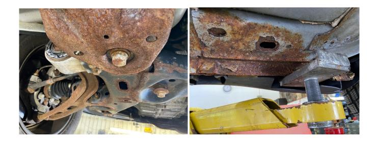
The underside of the vehicle body is showing considerable rust.
