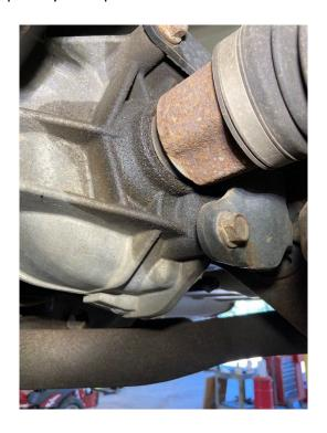
One of the axle seals on the rear differential is leaking and in need of replacement.
