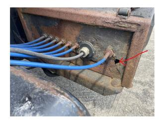
The valve box that contains the expensive hydraulic valves for all of the snow plow hydraulics is extremely rusty and has holes in it. These holes allow dirt, debris and salt to get on to the expensive hydraulic components. The metal is too rusty to attempt to weld/repair and the entire valve box would need to be replaced.
